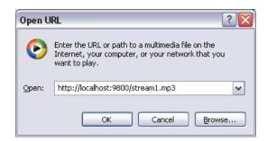
Enter the IP and port, then the stream name. Because the player is running on the same machine as the server in this case, 'localhost' is entered as the IP number. Were you to be listening on a another machine, you would enter the server's IP number, like this: http://198.168.1.107:9800/stream1.mp3. The stream name is the one that was configured in the steamcast.conf file. Click OK.
